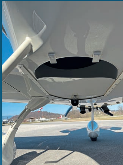
▲ Intriguingly, the test aircraft sported a non-standard belly camera port with a sliding cover
