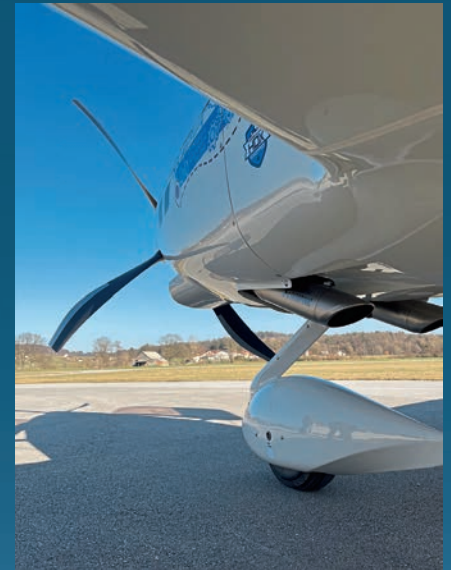
▲ Large diameter pipes give an idea of the typically high turbine gas flow. Nosewheel free-casters
