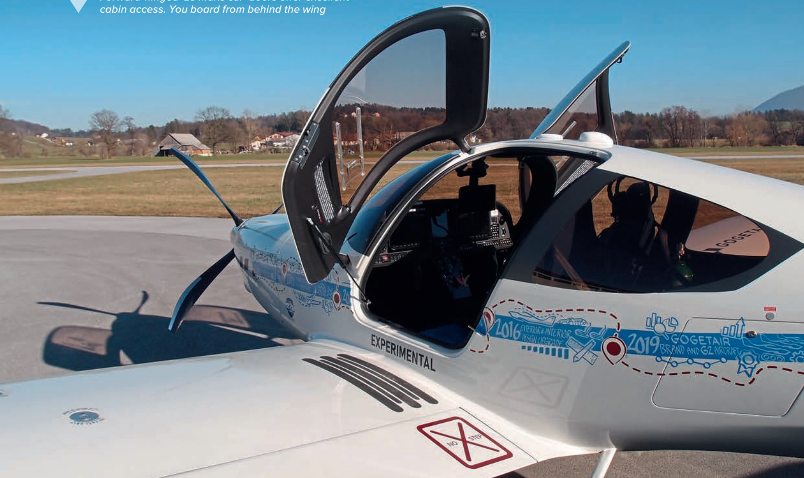
▼ Forward-hinged 'Le Mans car' doors offer excellent cabin access. You board from behind the wing
