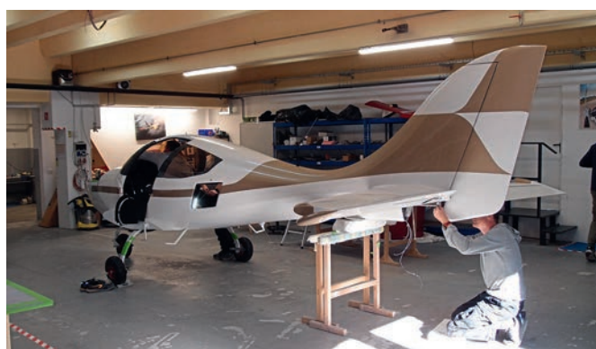
▲ G750s under construction at GOGETAIR's factory, located at Slovenske Konjice airport, near Loe. Note the baggage bay door and very different nose profile of these, the piston-engine model from which the G750TP turboprop was developed
