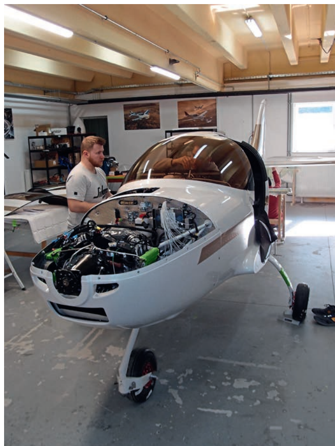
▲ G750s under construction at GOGETAIR's factory, located at Slovenske Konjice airport, near Loe. Note the baggage bay door and very different nose profile of these, the piston-engine model from which the G750TP turboprop was developed
